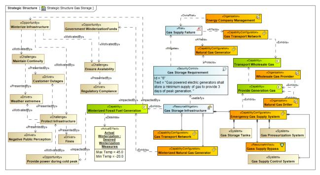
Figure 13 – Emergency Gas Storage System and Supporting Infrastructure
