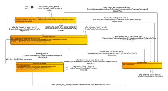
Figure 24. Search Region of Drone MSAR Control Software.
