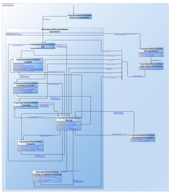
Figure 10. Logical State Machine for the Transporter
