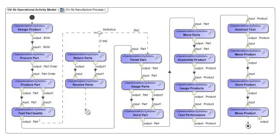
Figure 5. Manufacture Process Operational Activity Diagram
