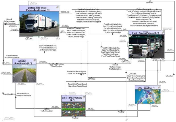
Figure 10: Truck Platooning Operational Connectivity
