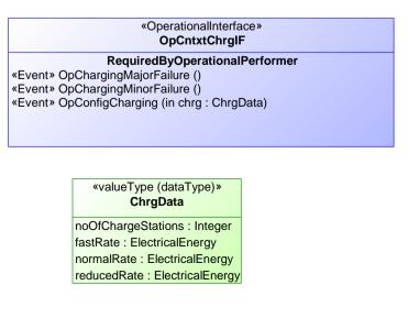
Figure 9. The interface between supervision and control and charging
